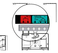
Use the ink provided to connect terminals 5 & 6 if no safety brake is required.
