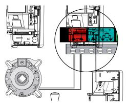
Connect the safety brake into terminals 5 & 6.
