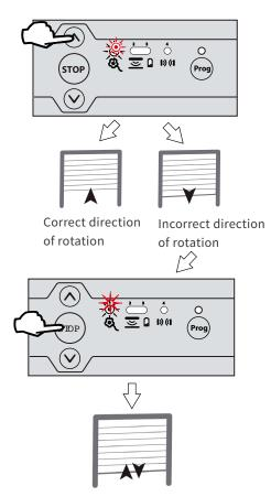
Briefly press the PROG button until the door jogs to complete the motor set up procedure. The motor & safety brake LED goes out and the safety edge LED comes on.
